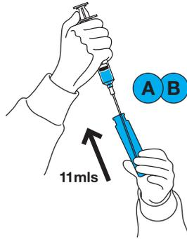
Aspirate **11mls** of "C" into the the second 20ml syringe using the second mixing cannula.
